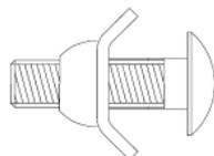
M8 x 30 Bolt, Shear Nut & Security Washer
